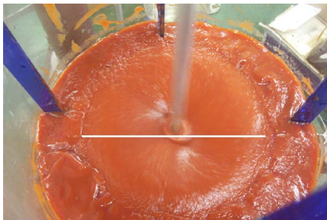
Fig. 5. Example of cavern diameter for ketchup with top exposed (the baffles are not necessary).
