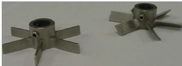
Fig. 4. Photograph of the straight and pitched impellers used in the study.
